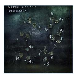
Thickness 23 mm Weight 54 kg Dragunov 7,62x54 API LIV. 3 AEP55
